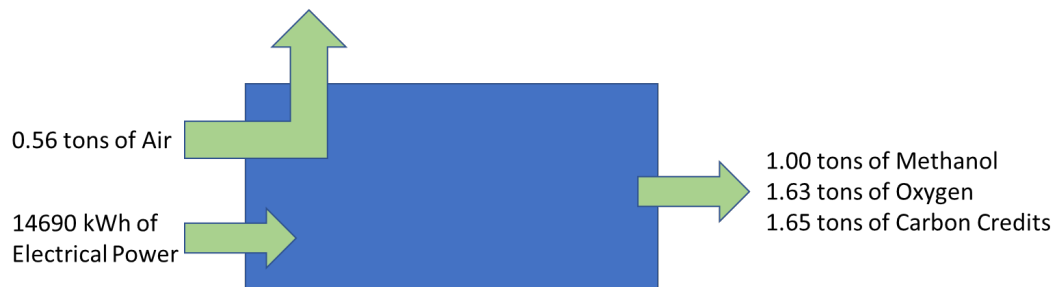
Figure 7: Overview of the Atmospheric Methanol Process
